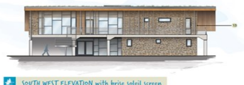
SOUTH WEST ELEVATION with brise soleil screen
